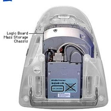
Remove the two screws at the top of the logic board/mass storage chassis and disconnect the cables and screw clamp.
