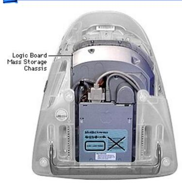
8. Remove the two screws at the top of the logic board/mass storage chassis and disconnect the cables and screw clamp.
