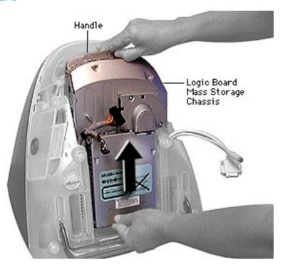
3. Using the handle, pull the main logic board/ mass storage chassis from the unit.
