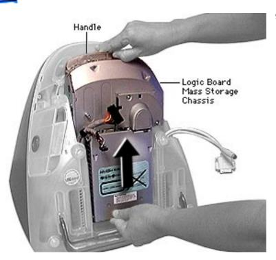
Using the handle, pull the main logic board/ mass storage chassis from the unit.
